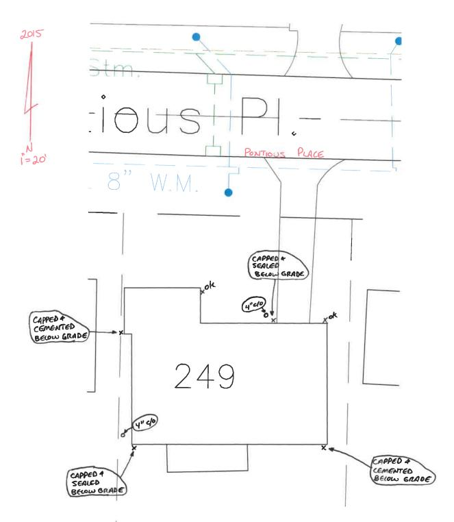
Investigation of illegal sewer connections revealed four (4) illegal connections. All downspouts have been corrected and are in compliance at this time.
